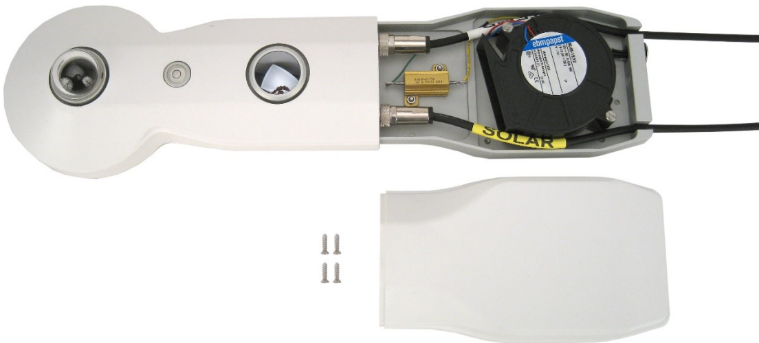
Figure C-4. CNF4 solar shield and four flat-head screws
