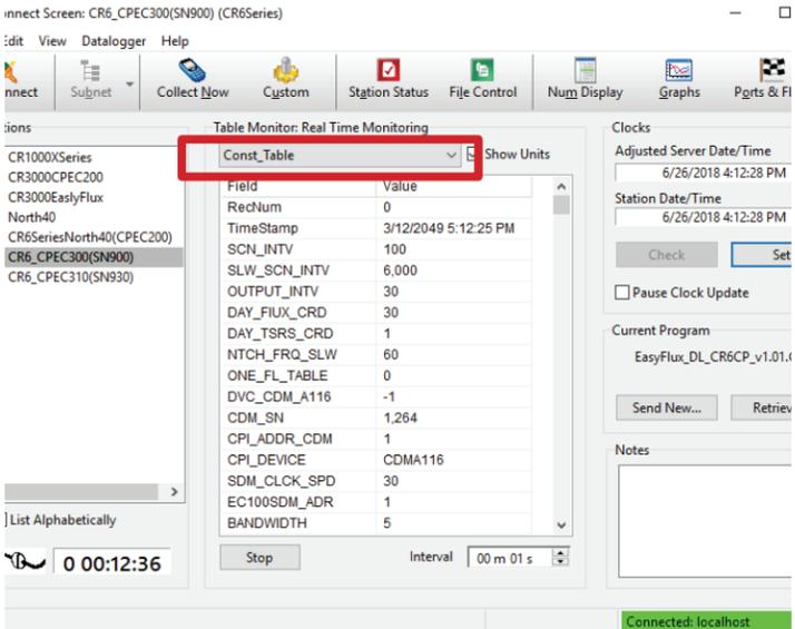
3. Confirm all the sensors used at the site are set to -1. To change a value in this table, right-click on the current value and select **View/Modify** from the pop-up menu. Press **Apply** once the new value has been entered.
