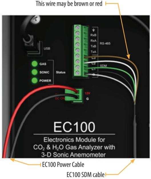
Draw the EC100 power cable and EC100 SDM cable through the feedthrough at the bottom of the CPEC306 enclosure and connect them to the DINrail.
