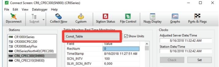
3. Confirm all the sensors used at the site are set to -1. To change a value in this table, right-click on the current value and select **View/Modify** from the pop-up menu. Press **Apply** once the new value has been entered.
