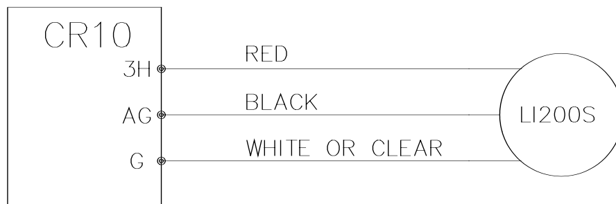
FIGURE 7.1-1. Wiring Diagram for LI200S
