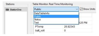
*PC400* users, click **Connect** <sup>\*</sup>, then **Monitor Data**. When this tab is first opened for a data logger, values from the **Public** table are displayed. To view data from other tables, click **Add ±**, select a table or field from the list, then drag it into a cell on the **Monitor Data** tab.
