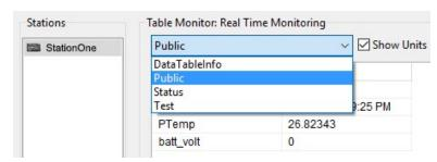
**PC400** users, click **Connect** , then **Monitor Data**. When this tab is first opened for a data logger, values from the **Public** table are displayed. To view data from other tables, click **Add** , select a table or field from the list, then drag it into a cell on the **Monitor Data** tab.
