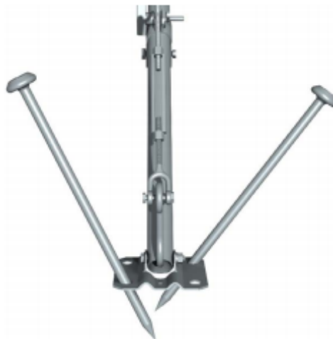
Figure C-2. Staking the tripod feet
