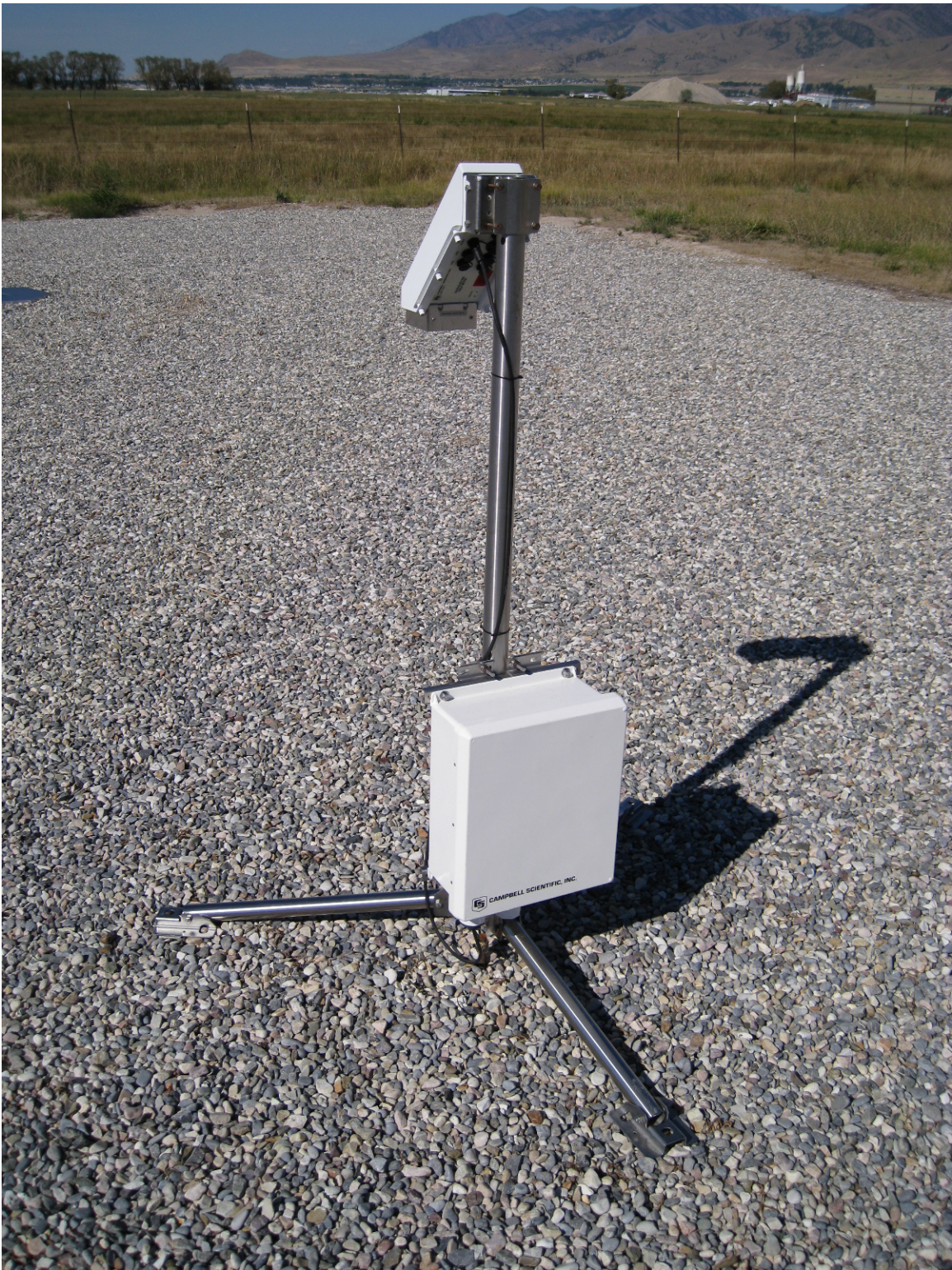
Figure J-1. Transfer Standard CS110 on CM310/CM350 at 1.2 meters
