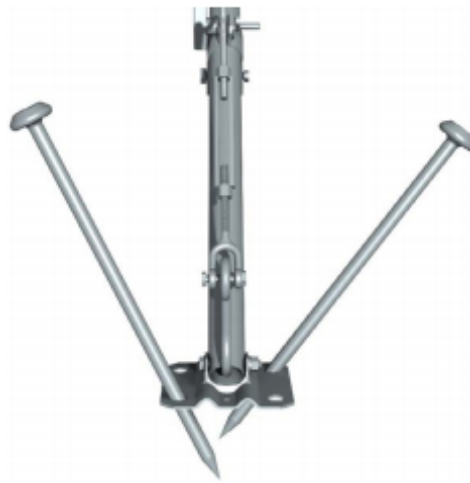
Figure B-2. Staking the tripod feet
