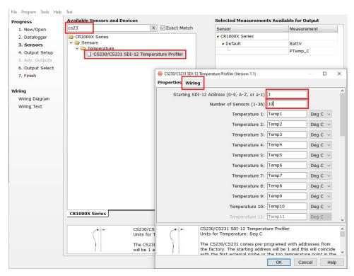
4. Click the **Wiring** tab to see how the sensor is to be wired to the data logger. Click **OK** after wiring the sensor.
