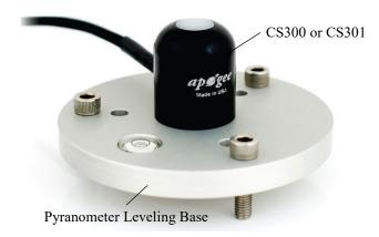
4. Loosely mount the pyranometer leveling base on the CM225 or 015ARM. Do not fully tighten the three mounting screws.
