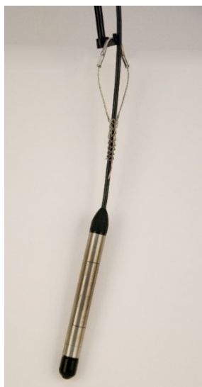
Figure 7-1. Transducer suspended with split mesh cable grip
