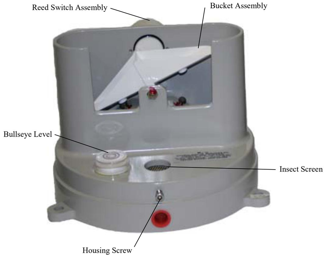
FIGURE 9-1. Components of CS700 Base
