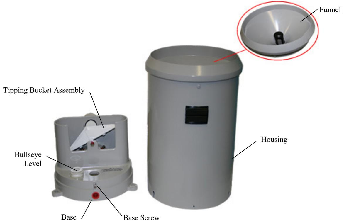
FIGURE 7-5. Main Components of the CS700
