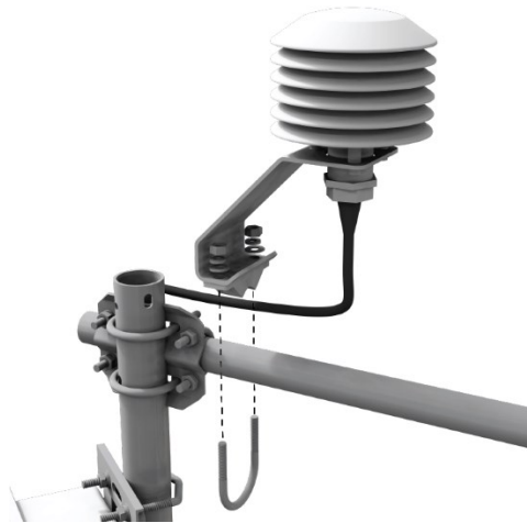
Figure 6-5. Mounting the temperature/relative humidity probe
