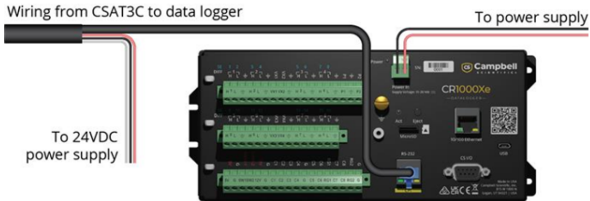
Figure 6-13. CPI connection to a CR1000Xe data logger with power connected to 24Vdc power supply
