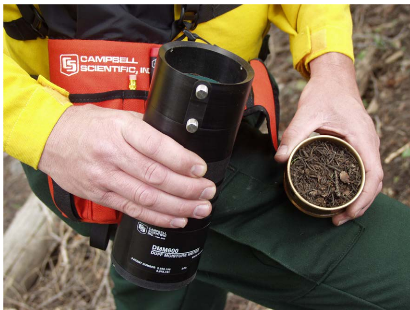
FIGURE 4-2. Duff placed in sieve
