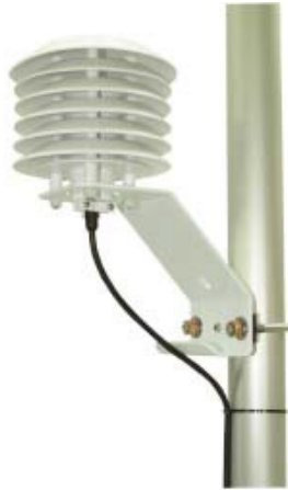
FIGURE 6-11. Solar radiation shield with EC150 temperature probe
