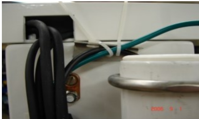
FIGURE 6-28. Loosely wire tie antenna cable
