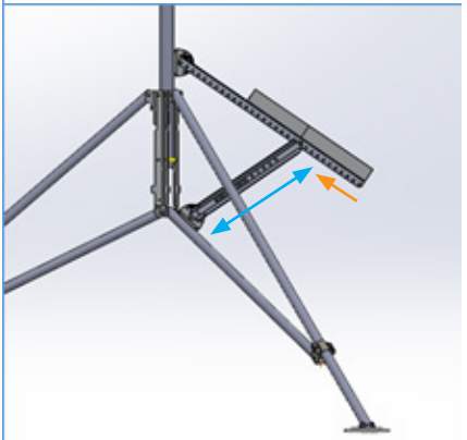
Figure 8: 0 degree to 35 degree mounting angles.
