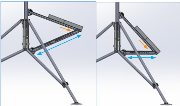
Figure 9: 20 degree to 50 degree mounting angles.
