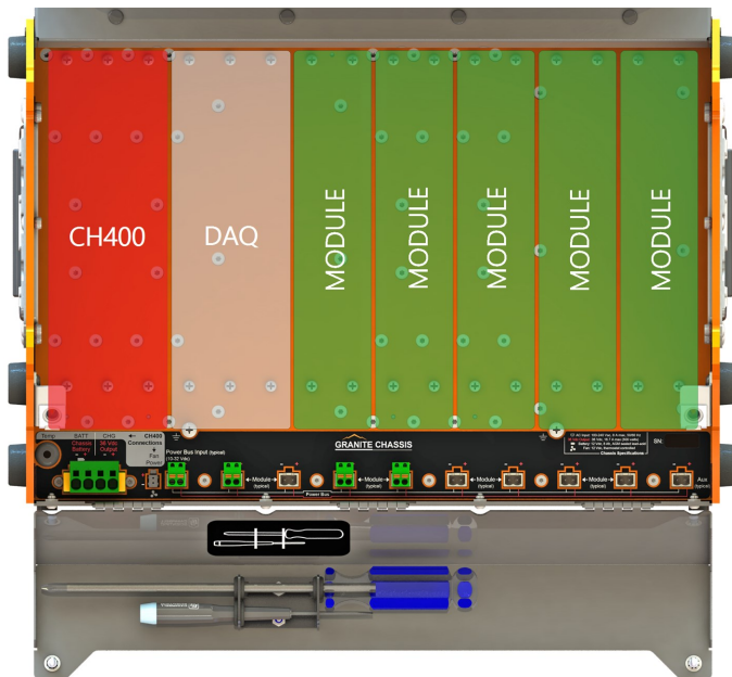
Figure 7-1. Typical module mounting locations
