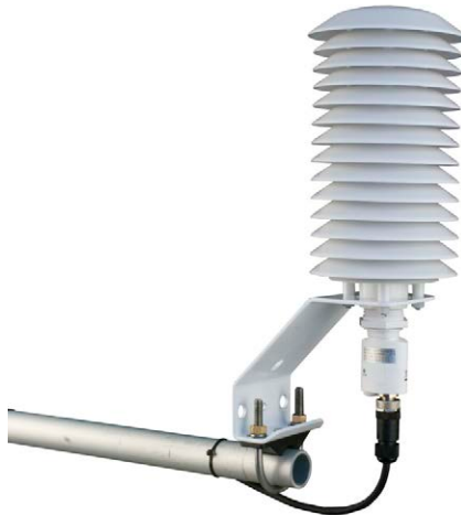
FIGURE 7-6. HMP155A and 41005-5 14-plate radiation shield on a CM200-series crossarm
