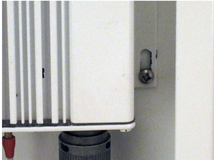
FIGURE 2. Proper mounting position of the electronics box.
