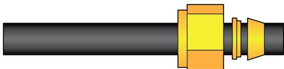
10. Hand tighten the cap and mark its location on the threads, and then tighten it another three quarters turn. Use a 5/8-inch wrench at the fitting base next to the enclosure to keep it from spinning while using an 11/16-inch wrench to tighten the cap three quarters turn. The three quarters turn should only be performed on the initial installation. See the following caution statement if reinstalling.
