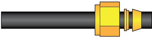
5. Hand tighten the cap and mark its location on the threads, and then tighten it another three quarters turn. Use a 5/8-inch wrench at the fitting base next to the enclosure to keep it from spinning while using an 11/16-inch wrench to tighten the cap three quarters turn. The three quarters turn should only be performed on the initial installation. See the following caution statement if reinstalling.
