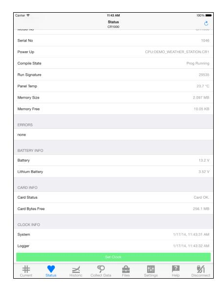
Note that a red E on the Status icon indicates that the datalogger has errors. Scroll down on the Status screen to identify the error. You can press the Reset button next to the indicated error to reset the value to 0.
