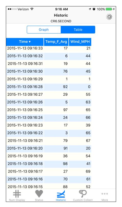
The data displayed on the **Historic** page comes directly from the datalogger and is "cloned" on the PC running *LoggerNet*. It does
