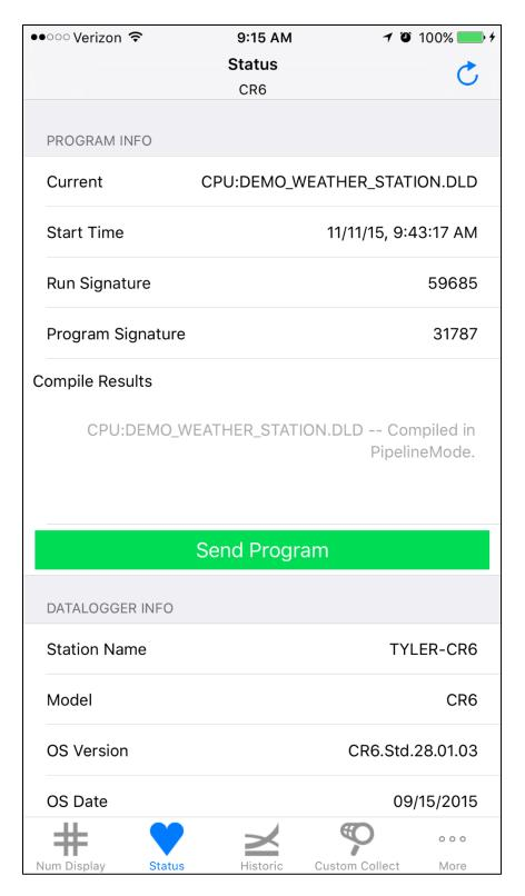
Note that a red E on the **Status** icon indicates that the datalogger has errors. Scroll down on the **Status** screen to identify the error.
