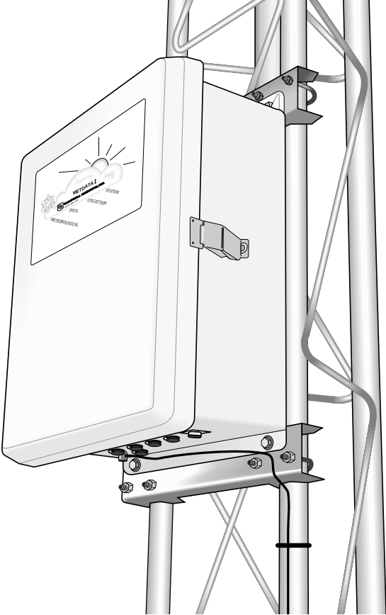
FIGURE 3.1-2. MetData1 Enclosure on UT10 or UT30 Tower
