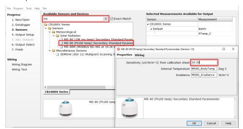
4. Click the **Wiring** tab to see how the sensor is to be wired to the data logger and 3WHB10K; a completion resistor such as the 3WHB10K is required to connect the MS-80 to a data logger. Click **OK** after wiring the sensor.
