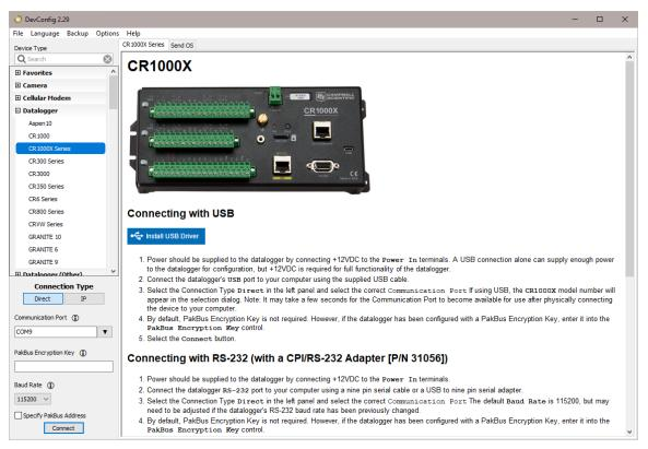
The DevConfig window is divided into two main sections: the device selection panel on the left side and tabs on the right side. After choosing a device on the left, you will then have a list of the serial ports (COM1, COM2, etc.) installed on your PC.
