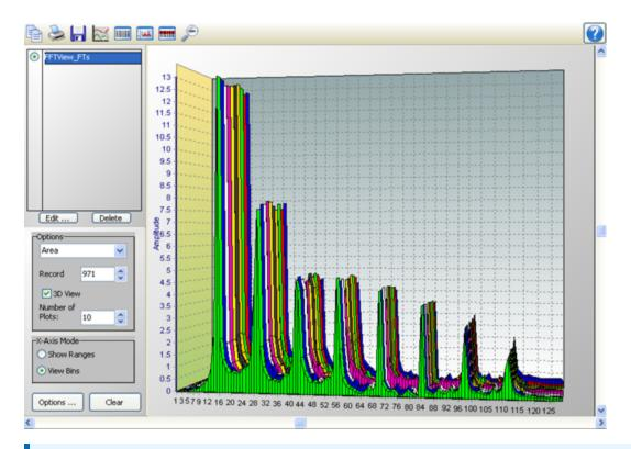
**NOTE:** View Pro does not create FFT data from time series information. It only displays FFT data contained in a \*.DAT file. FFT data in a \*.DAT file is created by using the CRBasic FFT instruction in a CRBasic program Data Table.
