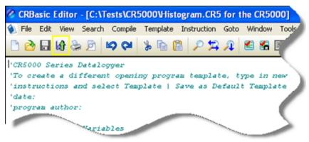
**NOTE:** When a file is sent to the datalogger using Compile, Save, and Send and the software is not actively connected to the datalogger, the software connects to the datalogger, sends the file, retrieves table definitions, and then disconnects. There will be little indication in the software that a connection was established.
