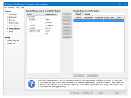
On the left, Short Cut will show the sensors you've added to be measured, with the measurement labels you've used. On the right is a multi-tabbed grid that shows the output tables.
