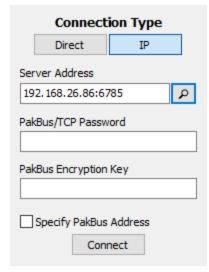
If the device supports IP communication, the **IP** button will be enabled. In order to communicate via IP, click **IP** under **Connection Type** and enter the IP address or domain name for the device in
