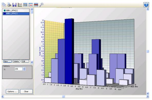
**NOTE:** View Pro does not create rainflow histogram data from time series information. It only displays rainflow histogram data contained in a \*.DAT file. Rainflow histogram data in a \*.DAT file is created by using the CRBasic Rainflow instruction in a CRBasic program Data Table.
