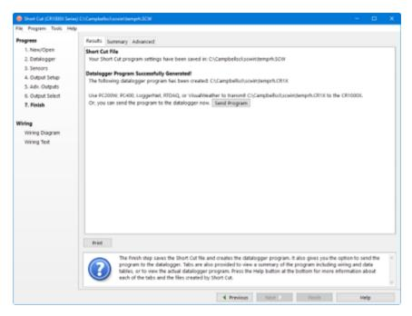
The **Results** tab provides information on the files that were created. If a program was created successfully, a **Send Program** button will also be displayed which allows you to send the program to the datalogger.
