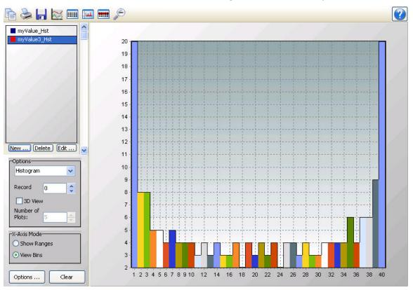
**NOTE:** View Pro does not create histogram data from time series information. It only displays histogram data contained in a \*.DAT file. Histogram data in a \*.DAT file is created by using the CRBasic Histogram instruction in a CRBasic program Data Table.
