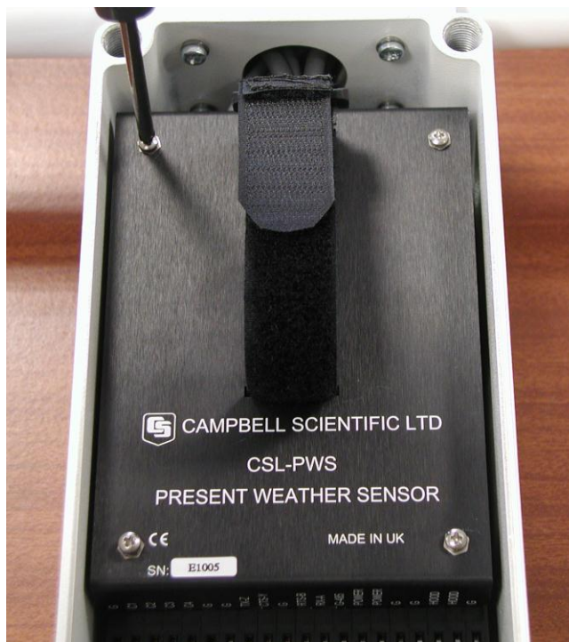
Figure 3-10. Removal of DSP cover
