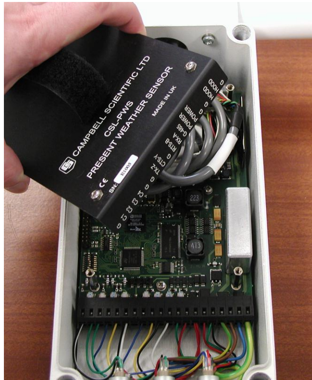
Figure 3-11. Exposing the DSP board
