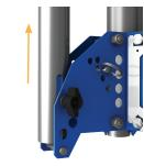
3. Rotate the leg down until the notch on the end of the leg lines up with the removable pin in the tripod frame. Slide the leg onto the pin until the notch is fully engaged with the pin.
