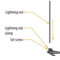
2. Place the lightning rod over the top collar, sliding it on until there is approximately 1.25 cm (1/2 in) of clearance between the top of the U-bolt and top of
