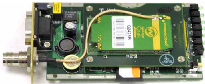
FIGURE B-6. Inserting the SIM
