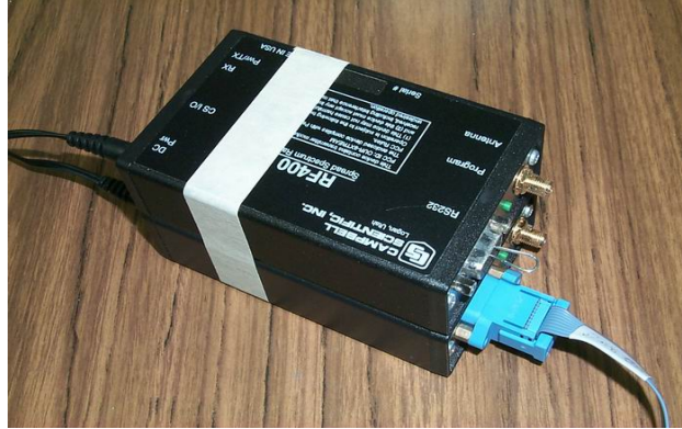
FIGURE K-1. Loop-back Test without Antennas
