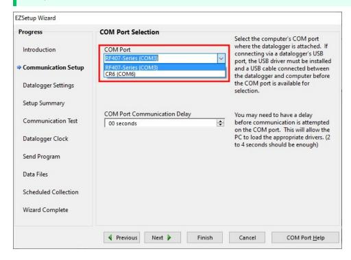
9. Accept the default value of **00 seconds** in the **COM Port Communication Delay** - this box is used to allow time for hardware devices to "wake up" and negotiate a communications link. Click **Next**.
