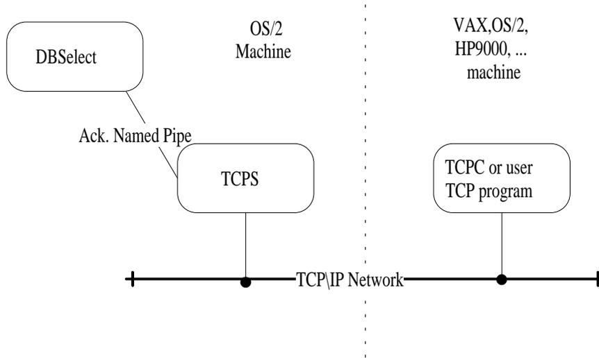
FIGURE 7-1. Example Named Pipe Client Software for TCP/IP Use
