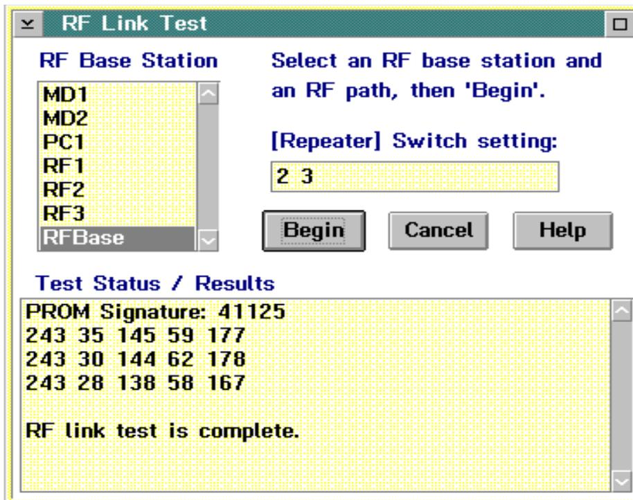
FIGURE 5-6. Radio Link Test View
