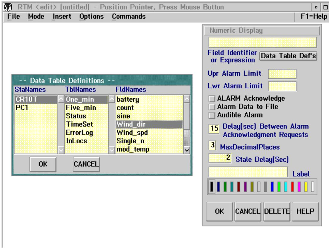
FIGURE 6-2. RTM Screen Showing Station.Table.Field for a Numeric Display
