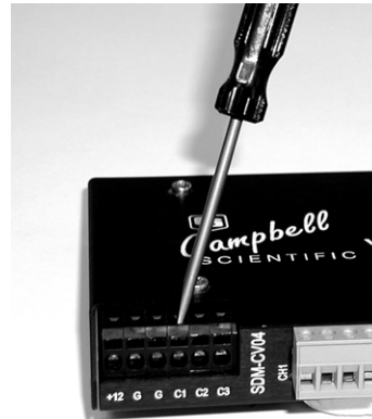
FIGURE 4-1. Use of the Spring-Loaded Terminal Blocks (Top Position)
