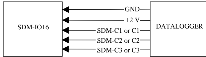
a) Connection with Datalogger Supply
