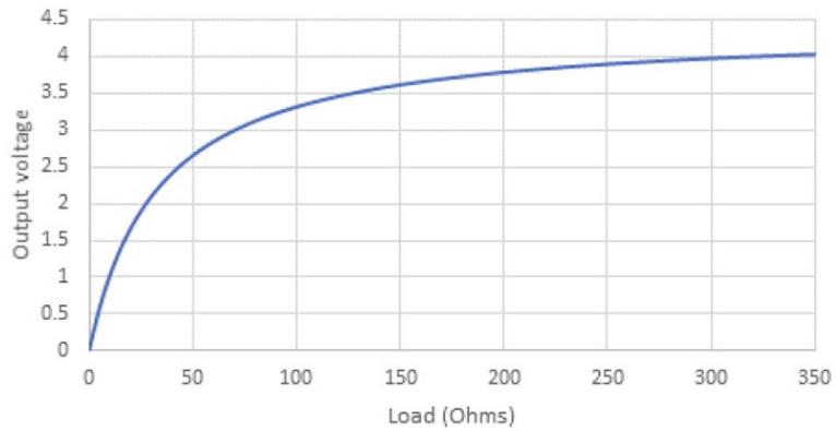
(e) Output voltage versus resistive load
