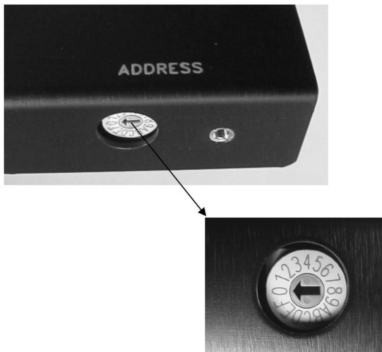
FIGURE 3-3. Address selection switch
