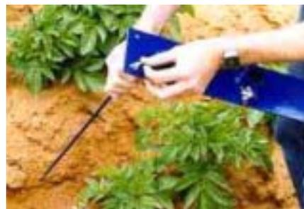
2. Place the assembled *stabilization plate* on the ground directly above the required position of the *probe*.
