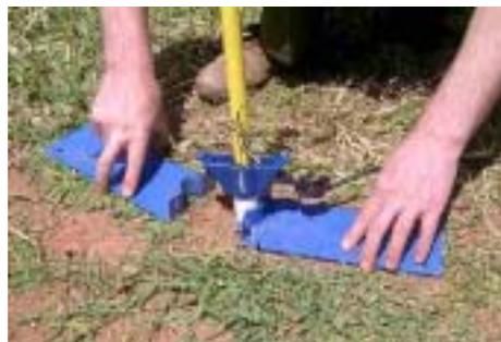
8. Continue inserting the probe into the ground with **gentle** blows of the *sledgehammer* using the *EasyAG 50 dolly*, until the base of the *top cap* is level with the ground. This will place the top *sensor* at 10 cm (3.9 inches) below the ground surface. Remove the EasyAG 50 dolly.
