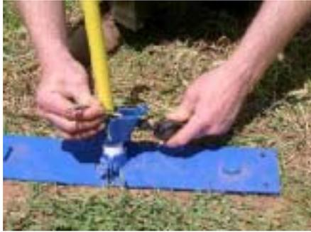
6. Remove the *stabilization plate wing nuts*.
