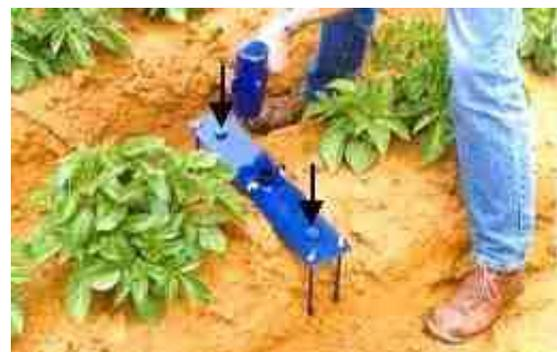
5. The *stabilization plate* should be firm to the ground without causing significant soil compression
