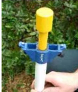
5. Continue inserting the *probe* by hammering on the insertion dolly with a *sledgehammer* until there is a 2.5 cm (1 inch) gap between the base of the *top cap* and the edge of the *stabilization plate tube* guide.
