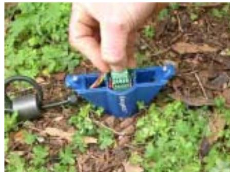
2. Pull the excess cable back through the *cabl e gland*. The outer sheath of the cable should be trimmed back as far as the point where the cable enters the inside of the top cap. Apply silicone around the wires of the cable at the end of the outer sheath, to prevent moisture from traveling along the cable into the inside of the *top cap*.
