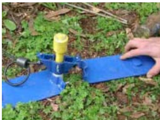
9. Continue inserting the probe into the ground with gentle blows of the *sledgehammer*, whilst holding the top of the probe steady with one hand, using the *EasyAG 80 dolly*, until the base of the *top cap* is level with the ground. This will place the top *sensor* at 10 cm (3.9 inches) below the ground surface. Remove the *EasyAG 80 dolly*.
