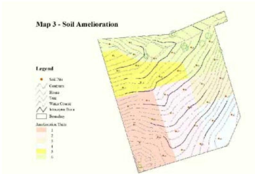
Once the soil has been ameliorated and improved then the altered soil properties are considered in conjunction with the topography, irrigation system and crop types to delineate irrigation management units.
