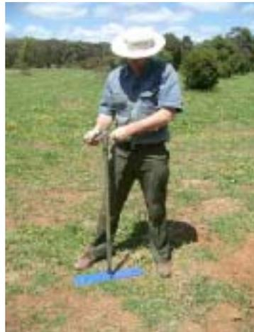
2. Using a *sledgehammer*, beat the *AMS soil sampler* into the ground until the bottom of the beating head sits 25 cm above the *stabilization plate*. **Note:** While it is preferable to go all the way in one insertion, successful installation may be possible in heavier soils with 2 insertions. Ensure accurate blows are made such that lateral deflection of the soil sampler is minimized.
