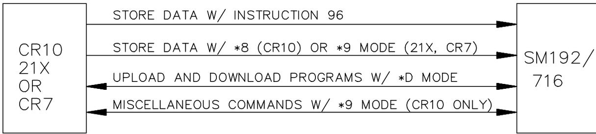
**Figure 1.4-1 Operation with Current CR10, 21X, and CR7**
