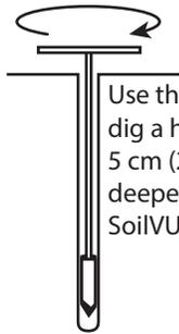
Use the auger to dig a hole about 5 cm (2 in) deeper than the SoilVUE length.
