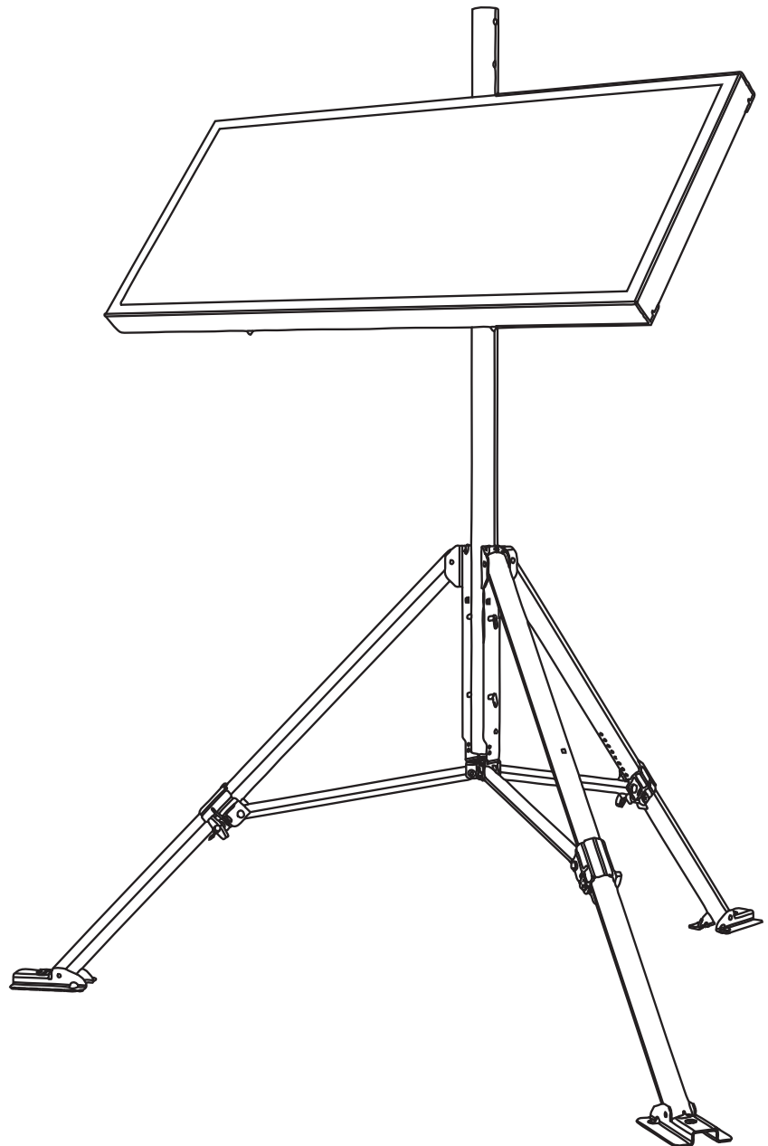
FIGURE 3-13. Solar panel mounted on a tripod. Panel can be mounted to the tripod leg.
