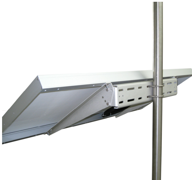
FIGURE 12. SP70 is Mounted to a Pole Using Two 5/16-18 x 2.0 U-Bolts
