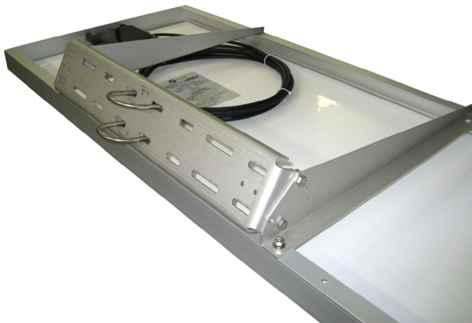
FIGURE 9. Two 5/16-18 x 2.0 U-Bolts are Used for Pole or Tripod Mounting
