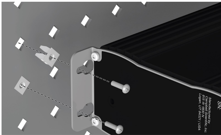
Figure 12-3. Enclosure backplate mounting
