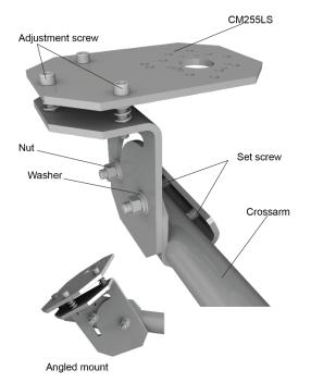
6. Verify mounting hardware is firmly tightened, and that the mounting bracket is at the desired angle.
