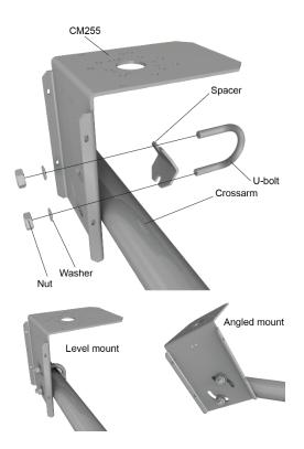
5. For pyranometers mounted horizontally, ensure the mounting bracket is horizontal in two dimensions. For pyranometers mounted at an angle, set the mounting bracket angle to the desired angle prior to tightening the mounting hardware.
