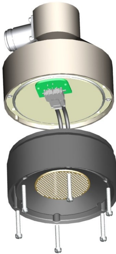
FIGURE 9-3. Remove transducer housing and disconnect wires
