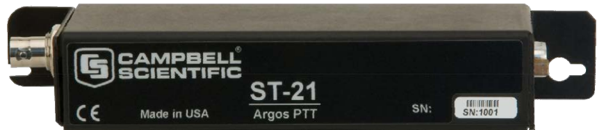
FIGURE 1-1. ST-21 Argos Satellite Transmitter
