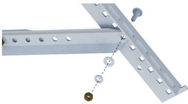
Figure 3-5. Attaching the support struts to the mount arms
