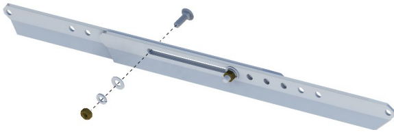
Figure 3-4. Assembling the support struts
