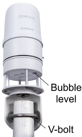
Figure 3-9. Bubble level on the ClimaVue 40
