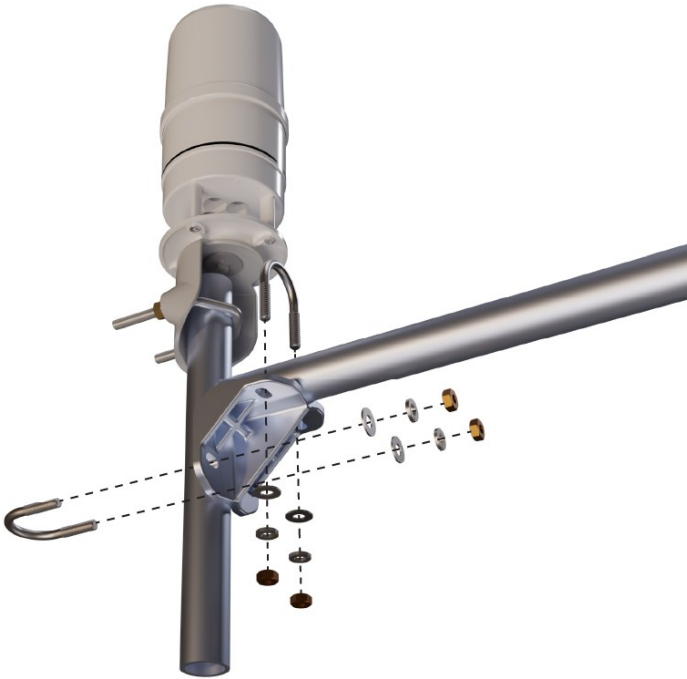
Figure 3-7. Mounting tube installation
