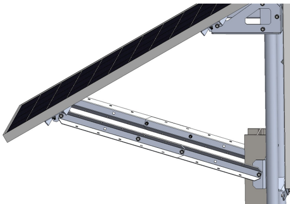
Figure 3-5. Solar panel at 30° angle
