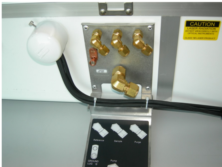
FIGURE 6-15. Routing of SDM and power cable through TGA200A feedthrough bracket
