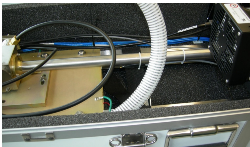
FIGURE I-2. Location of first thermistor probe attachment
