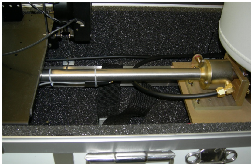
FIGURE I-3. Location of second thermistor probe attachment
