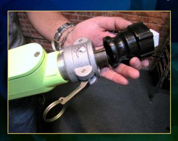
Remove the protective cap. Align the slot on the WEATHERPAK® with the guide pin on the quick release. Push straight in. (DO
