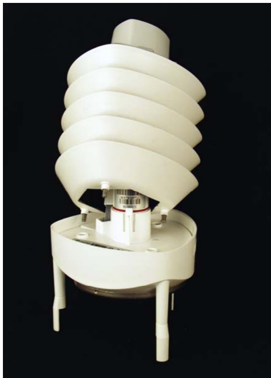
FIGURE 2. A WXT510 with the PTU inserted inside of it.
