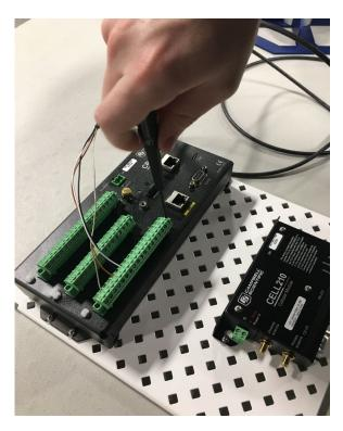
Plug ClimaVUE50 sensor cable into CR1000X datalogger
