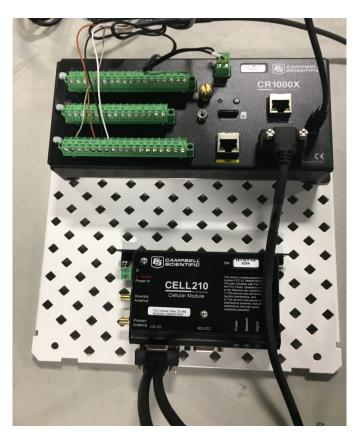
Install SC12 into CR1000X and cellular module
