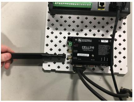
Install antenna into cellular module
